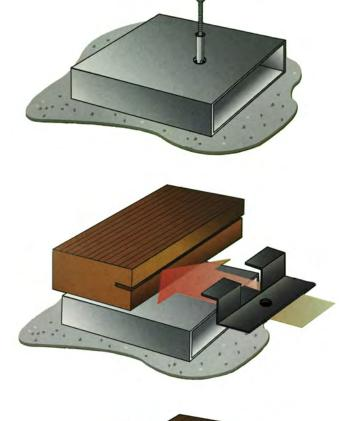
Our aluminium battens are held in place by 38mm Anchor bolts that secure onto the concrete surface below.
