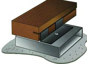
We then secure then plastic clip into the batten which in turn firmly holds the composite timber in place. This process is repeated to create a beautiful decking area with all screws and fasteners hidden away.
