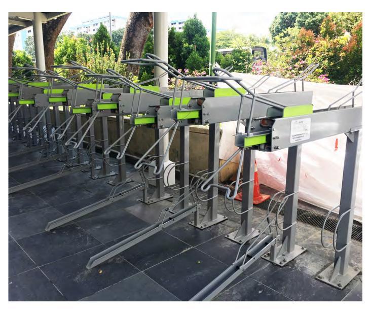
For when space is very limited we have our custom style staggered tier range. Usually we allow at least a 600mm gap between each rack to make sure neighboring bicycles do not collide, but using our staggered system you are able to shorten that gap to 450mm! By subsequently altering the height of rack to differ from the last, we can have each bicycle closer together without danger of them colliding.
