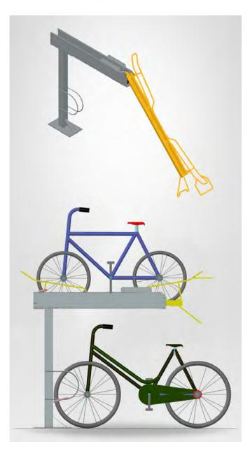
Our U series bicycle rack is our timeless series, first being installed at Pasir Ris station in 2006. Our racks are made completely of hot-dipped galvanized steel, this means steel dipped in a special zinc coating to improve it's resilience against rust and wear. It is then powder coated in grey to give it both a smooth finish and further protection against rain and sunshine.
