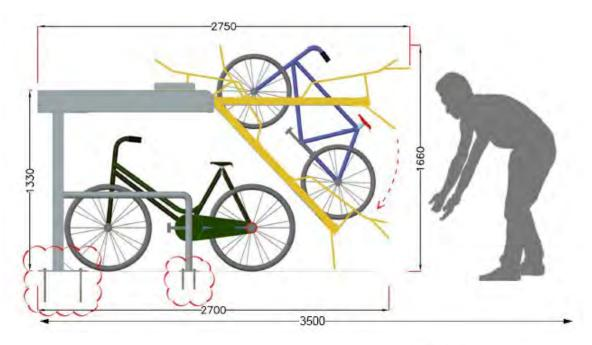
Additionally, Parkabikez must be installed with **650mm between the center of each bicycle rack** (650mm C/C). This allows space for adjacent handlebars and pedals to not clash with one another. For a closer space saving solution check out our staggered series on page 33.
