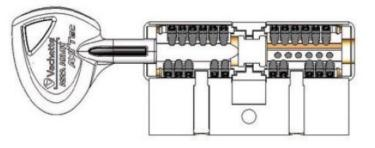
Double cylinder. 3 keys. Minimum dimension: 27.5 x 27.5 mm Nickel plated - Ref. 7011 AXI'TEC
