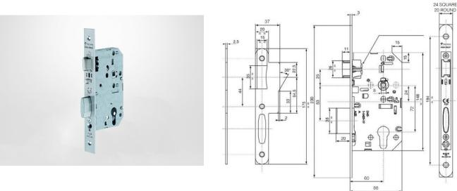
Same as D548 with snib on front plate that prevents from projecting the deadbolt when the door is not shut. NO RISK OF PREVENTING FIRE DOOR TO SHUT
