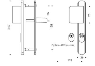
Escutcheon thickness 7 mm - Fixing centers 70 mm - Door Thickness 38 to 48 mm Ref. 534/1338L/6359
