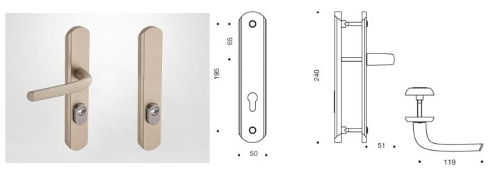
Wide Plate - Ref. 1338L/6349 **Narrow Plate** Escutcheon thickness 8 mm - Fixing centers 92 mm - Door thickness 58 to 68 mm - Ref 1338L/6359 Escutcheon thickness 7 mm - Fixing centers 70 mm - Door Thickness 38 to 48 mm - Ref. 338L/6359
