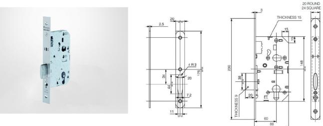
Deadlock for Euro-profile cylinder. Deadbolt 20mm projection, double throw. Front plate 20 mm rounded ends (R20) or 24 mm square ends (K24). Backset: 60 mm.
