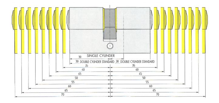
On request, Vachette cylinder can be supplied in extended version (for overlapping doors, extra thick doors, etc).
