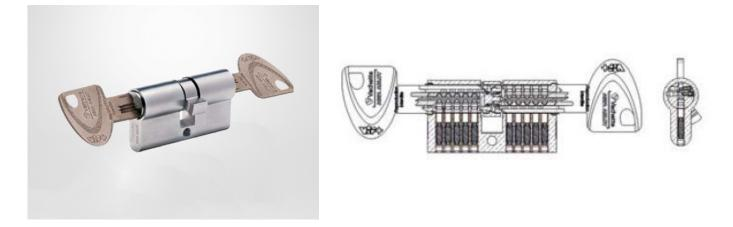
Double cylinder SYNKRO with emergency key function, characterised by nickel-plated cam. This function allows a door to be unlocked from either side even if a key is still inserted on the other side.
