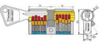
Double cylinder. 3 keys Minimum dimension: 30 x 30 mm Nickel plated Ref. 7101 Brass finish - Ref. 7100
