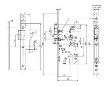
Classroom or office lock for Euro-profile cylinder. Equipped with anti-thrust bolt. Key to latch. Outside handle made inoperative when locked. Exit always free. European CE standards with 8 mm follower (C8), center to center 72 mm, Backset: 60 mm. Fire rated as standard.
