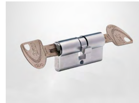
Double cylinder SYNKRO with emergency key function, characterised by nickel-plated cam. This function allows a door to be unlocked from either side even if a key is still inserted on the other side. 3 keys. Minimum dimension: 30 x 30 mm up to 70 x 70 mm. Nickel plated - Ref. FCS 7101 VIP+
