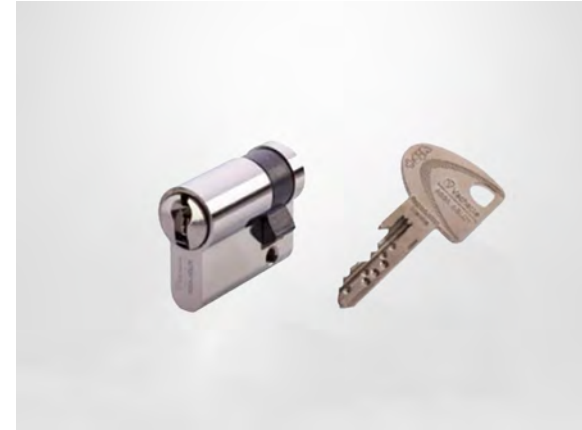
Single cylinder with adjustable cam. 3 keys Minimum dimension: 30 x 10 mm Nickel plated - Ref. 5101 VIP+
